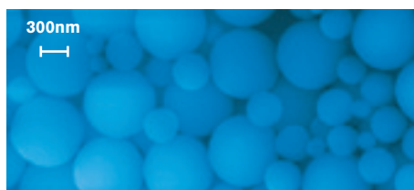
FIGURE 3B: SEM image of the polystyrene particle sample confirms the presence of three populations at around 220nm, 400nm and 780nm in diameter.
